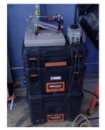
WJE also performed quality assurance field tests on mock-up installations as well as in-place commercial glazing systems (curtain wall) and fenestration products (window wall). These tests consisted of water penetration resistance testing and air infiltration testing. Water and Air Testing Observation Reports were issued throughout the construction phase that outlined WJE's observations, summarized the test results, and provided remedial recommendations for consideration by the project team.
