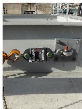
Each anchorage point was loaded in a manner that replicated the minimum design load (i.e., 5,000 pounds) required by OSHA and the Chicago Building Code in potential directions of use. The new equipment sustained the test load in an appropriately elastic manner and was certified for use.
