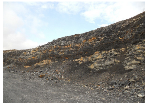
FIGURE 1. A PYRITIC SHALE FORMATION IS EXPOSED AT A QUARRY FACE. WITHIN THREE YEARS OF EXPOSURE, OXIDATION OF THE PYRITE HAS LED TO IRON OXIDE STAINING AND DEGRADATION OF THE SURROUNDING SHALE.
