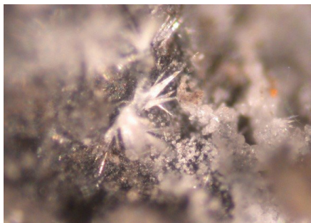
FIGURE 3. A MICROGRAPH OF GYPSUM CRYSTAL GROWTH WITHIN AN OPEN BEDDING PLANE IN THE SHALE PARTICLE.
