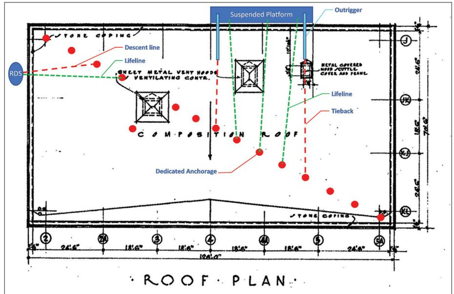
Fig. 4: Sample anchorage layout showing sample rigging configurations
