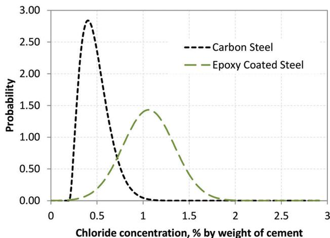
Fig. 6—Recommended probability distributions for chloride threshold for carbon steel-reinforcing bars and ECR.
