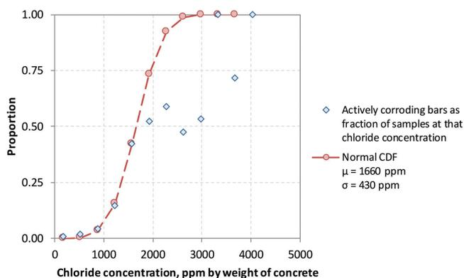
Fig. 5—Plot of actively corroding ECR as fraction of samples at that chloride concentration—an estimate of cumulative distribution of chloride threshold for ECR—versus chloride concentration at bar depth. Assumed normal cumulative distribution function (CDF) fit to data is also shown.
