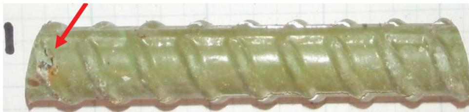
Fig. 3—Bar sample (core 2) from U.S. Route 30 Bridge<sup>27</sup> showing corrosion at preexisting damage site (arrow).
