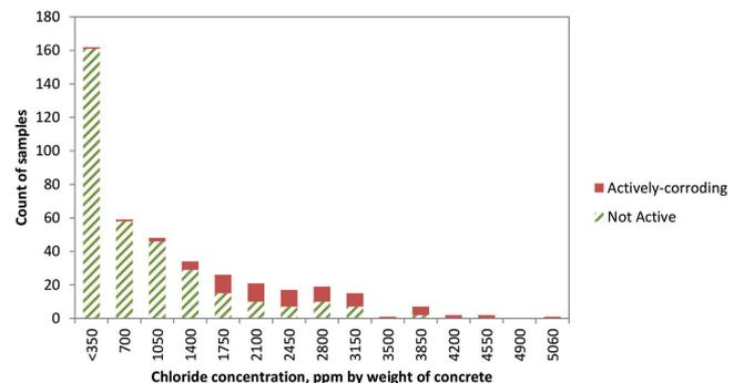
Fig. 4—Histogram of actively corroding versus nonactive extracted ECR samples from evaluated bridge decks and substructures.
