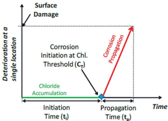
Fig. 1—Corrosion sequence (adapted from Tuutti<sup>2</sup>).
