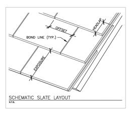
After repair work to underlying flashings and gutters, some contractors don't pay attention to these critical dimensions. The result is a slate roof that is more susceptible to water infiltration. Knowing what to look for is critical, as headlap and offset problems can be easy to overlook, especially if observations are made from a distance. Check out the following examples.
