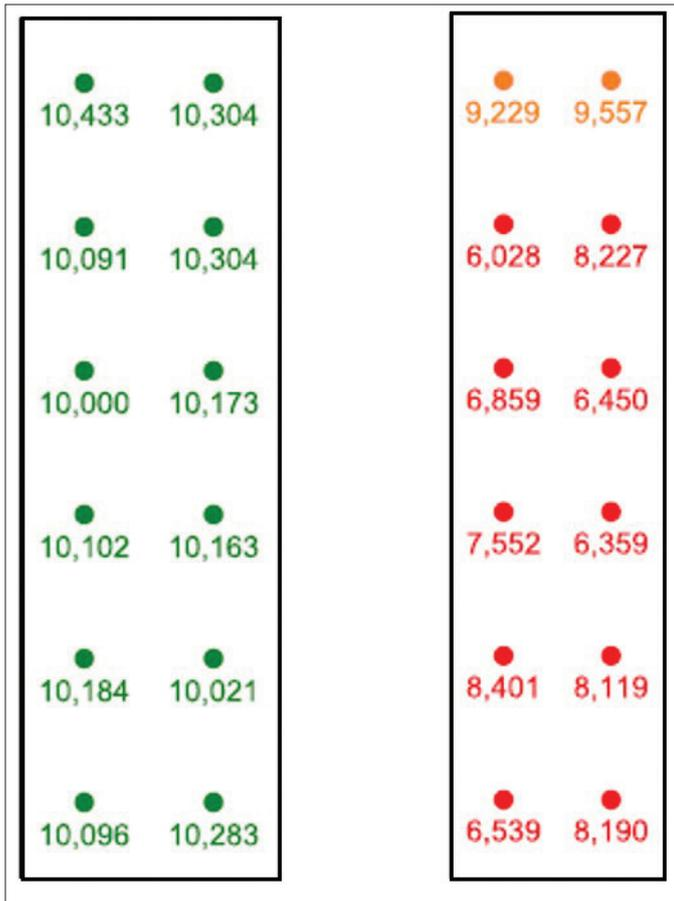
Fig. 7: Comparison of representative UPV material velocities (feet per second) for an undamaged concrete column (left image) and a damaged concrete column (right image)
