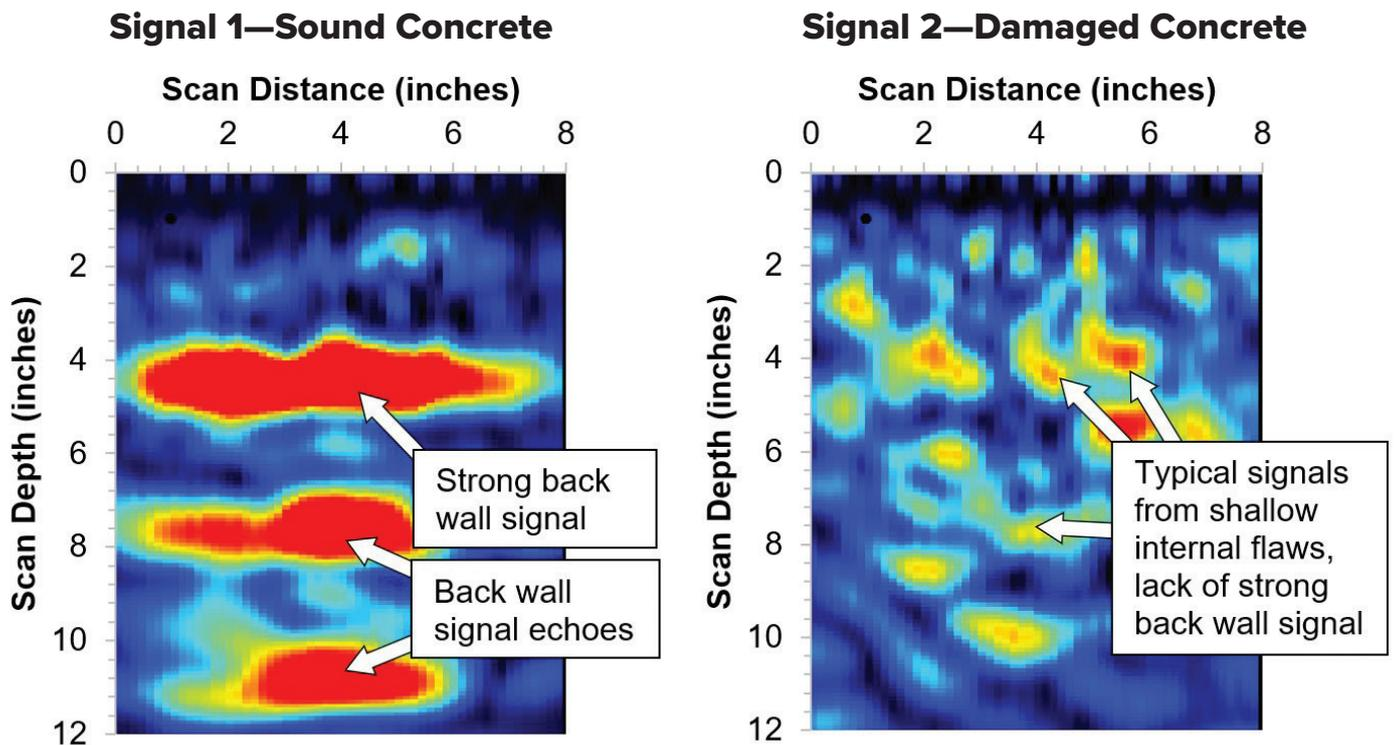
Fig. 6: Comparison of representative UST results in damaged and undamaged areas
