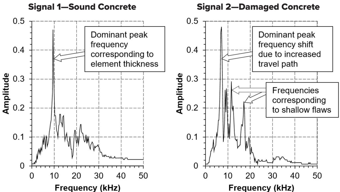
Fig. 5: Comparison of representative IE results in damaged and undamaged areas
