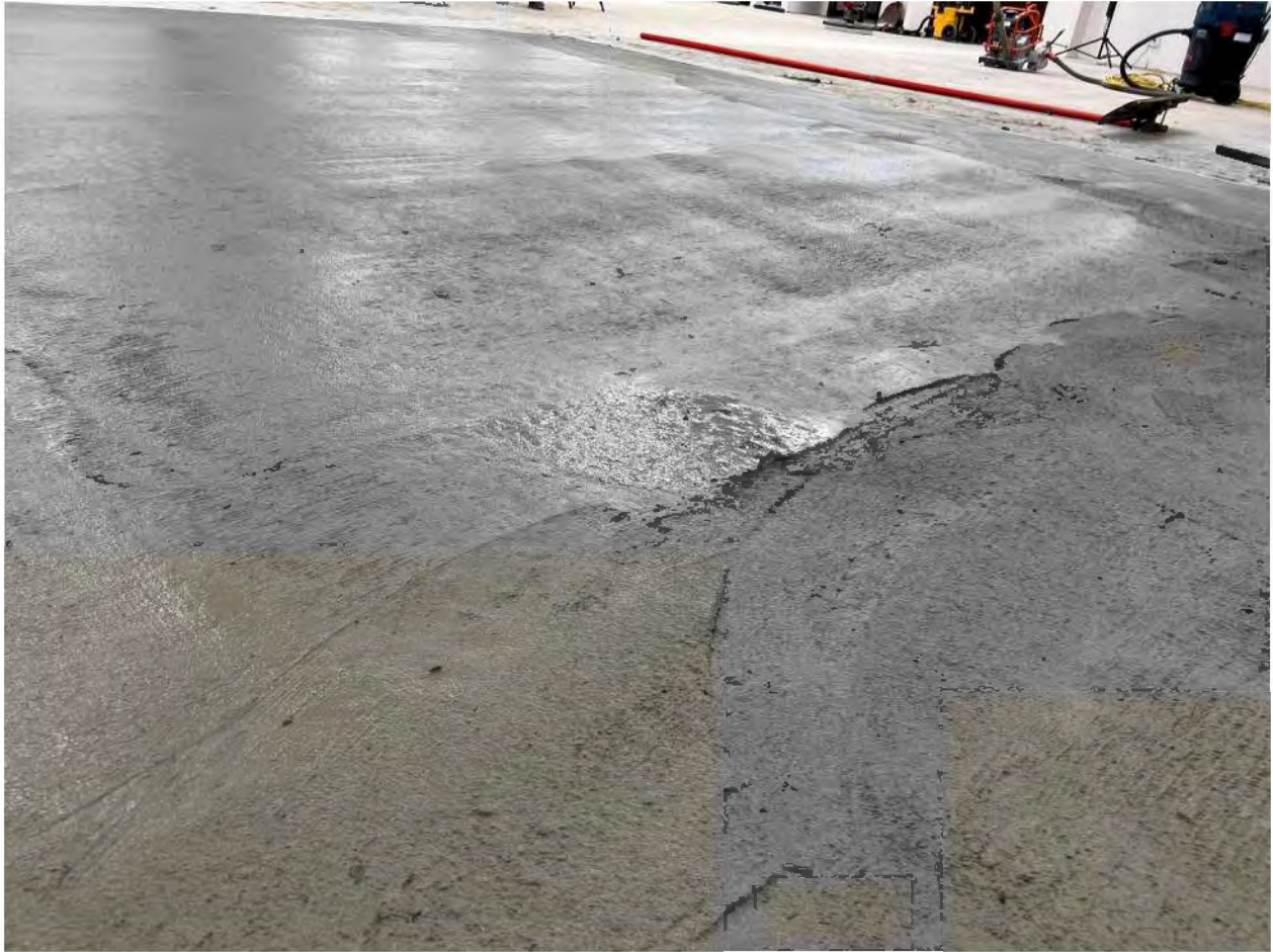
Figure 14. Slab 1, Mix 1 close-up photograph of concrete surface following bull floating and hand troweling at edges. Note small amount of bleed water.
