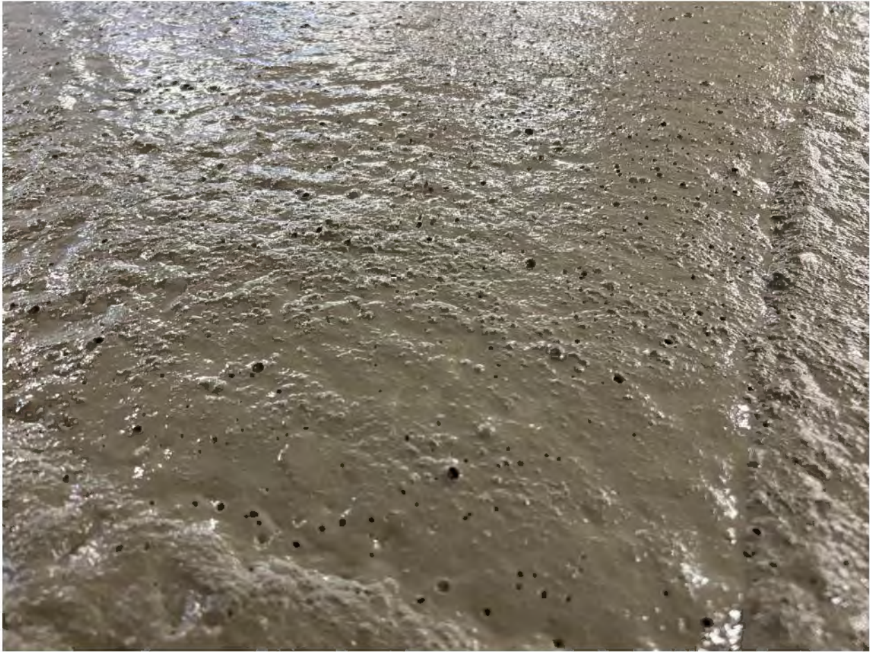
Figure 13. Slab 1, Mix 1 close-up photograph of concrete surface following vibratory screeding.
