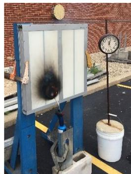
The translucent wall panels proposed for thirteen percent of the exterior walls provided a cost-effective enhancement to the architectural character of the center. Tests showed that the product had low flame spread and smoke development characteristics. This, coupled with enhanced sprinkler protection and strategic placement on the building exterior, yielded a fire safety risk within the bounds contemplated by the building code and was approved by the local authorities.
